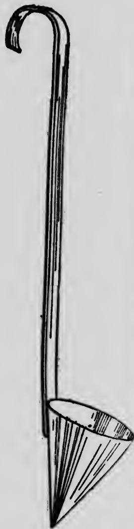
FIG 4. Six of these dippers full should just fill the sample bottle.
