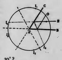
If objects are placed between the mirrors they form with the images a symmetrical pattern if the angle between the mirrors is a submultiple of 360°. The toy called the kaleidoscope is generally formed by placing coloured bodies between two mirrors at an angle of 36°, or between three mirrors forming an equilateral triangle.
