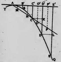
vals, E'E in 4, and so on. LE(=E'E-D'D) is the distance fallen in the fourth interval and represents the velocity at the middle (P') of this interval. If we mark P so that P'P = LE and points M, N, O, similarly, the curve AMNOP (a straight line) gives us the vertical velocity of the particle at each instant. It is called the velocity curve. Since the velocity increases uniformly the difference between two successive ordinates to this curve (as P'P = O'O) should be a constant, the acceleration.
