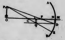
is called the focus. Usually only a small portion of a spherical surface is used as a mirror, so that CM is large compared to AM and NM.
