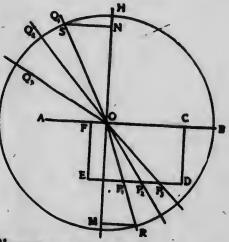
pendicular to AB. Place some pins as  $P_1$ ,  $P_2$ ,  $P_3$ , close to the edge of the block and place others, as  $Q_1$ ,  $Q_2$ ,  $Q_3$ , so that  $Q_1OP_1$ ,  $Q_2OP_3$ , etc., appear straight lines. Then  $Q_1OP_1$  is the path of a ray passing from air to glass,  $Q_1OH$  being the angle of incidence, and  $P_1OM$  the angle of refraction.
