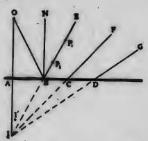
uprign by a little soft wax as the mirror, place two pins,  $P_1$  and  $P_2$  in line with the image *I*. Moving the eye to other points, *F* and *G*, find other lines in the same way and show that they all meet at a point *I*. Show also that *OI* is perpendicular to the mirror and bisected by it.
