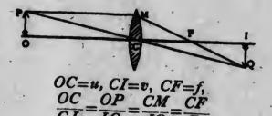
the same formula as for a mirror. We consider u + if the object is on the side of the lens from which the light comes, that is, if the object is real; v + if the image is on the side to which the light goes, that is, if the image is real. f is + if the lens is convex, - if it is concave.
