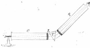
Fig. 62.—Course of rays through a spectroscope.
