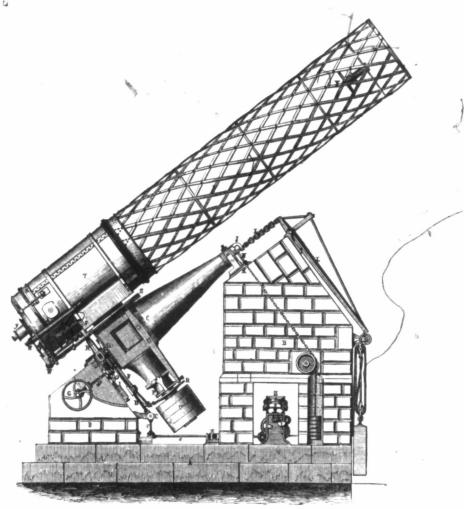
Fig. 43.—The great Melbourne reflector. T, the tube containing the great mirror near its lower end. Y, the small mirror throwing the light back to the eye-piece, y. C N, the polar axis. U, the counterpoise at the end of the declination axis. Z, the clock-work which moves the telescope by the jointed rods z e e E, and the clamp F.
