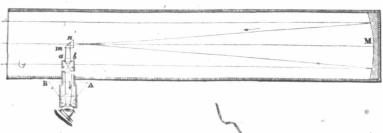
Fig. 37.—Horizontal section of a Newtonian telescope. This section shows how the luminous rays reflected from the parabolic mirror M meet a small rectangular prism m n, which replaces the inclined plane mirror used in the old form of Newtonian telescope. After undergoing a total reflection from m n, the rays form at a b a very small image of the heavenly body.
