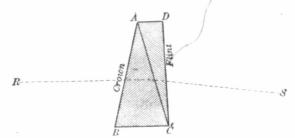
Fig. 31.—Refraction through a compound prism.
