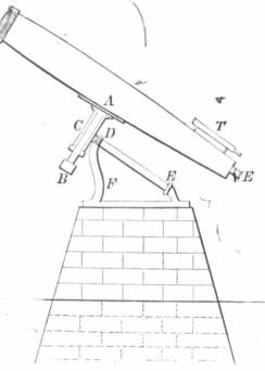
Fig. 34.—Mode of mounting a telescope so as to follow a star in its diurnal motion.
