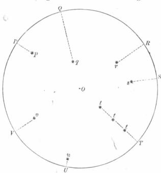
Fig. 1.—Section of the imaginary celestial sphere. The observer at O, looking at the stars or other bodies, marked p, q, r, s, t, u, v, will imagine them situated at P, Q, R, S, T, U, V, on the surface of the sphere, where they will appear projected along the straight pP, qQ, etc.
