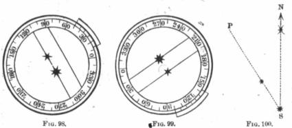
which the direction of one star from another is reckoned is this: Imagine a line, SN, in Fig. 100, drawn due north from the brighter star, and another, SP, drawn through the smaller star. Then the angle NSP which these two lines make with each other, counted from north towards east, is the position angle of the stars, the changes in which show the revolution of one star around the other.
