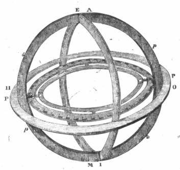
Fig. 27.—Armillary sphere, as described by Ptolemy, and used by him and by Hipparchus. The circle EI is set in the plane of the ecliptic, the line PP being directed towards its pole. The circle ApMp passes through the poles of both the ecliptic and the equator. The inner pair of circles turn on the axis PP, and are furnished with sights which may be directed on the object to be observed. The latitude and longitude of the object are then read off by the position of the circles.
