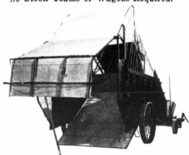
This cut shows bottom tilted and the end door partly opened, showing method of dumping load and the feeder.
