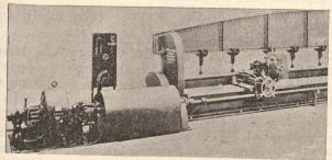
and running at slow speed, which furnishes ample power to enable the machine to plane two-inch armor plate, taking a heavy chip. The saddle of the planer is designed to carry two tools, one cutting in each direction, also a third tool for vertical feed, the saddle and tool holder being shifted automatically at any point desired.
