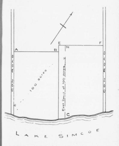
Mr. Niven—I would divide the lot into north and south halves by measurement, connecting B and E by a straight line, then I would divide the four equally in area.
