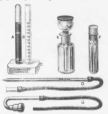
Fig. 22.-Haldane's Modification of Gowers' Hæmoglobinometer.
