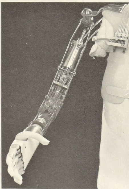
All movements of the first hydraulic arms were controlled by a lever near the shoulder.
