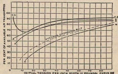
Curve 13, showing percentages of power transmitted by the different treated belts at different tensions, by taking 100% as the total amount (see page 28) capable of being transmitted.
