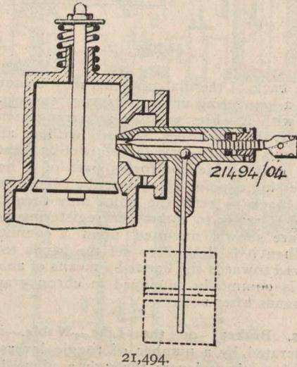
having been intimately penetrated by a current of air, this spray is volatilized by the heated surfaces and then fed to the motor.
