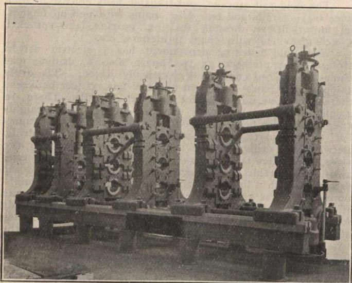
Roll Housings Assembled in Shop on Temporary Shoe Plates.
