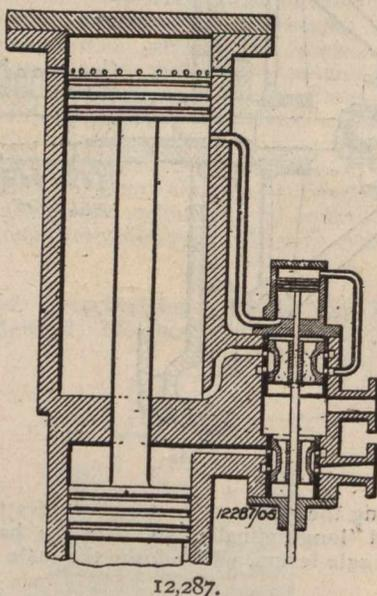
has heretofore been necessary where a number of repeated blows was desired, to move the lever at each stroke. By the present invention such lever may be switched out of action, and the hammer caused to work automatically and continuously.
