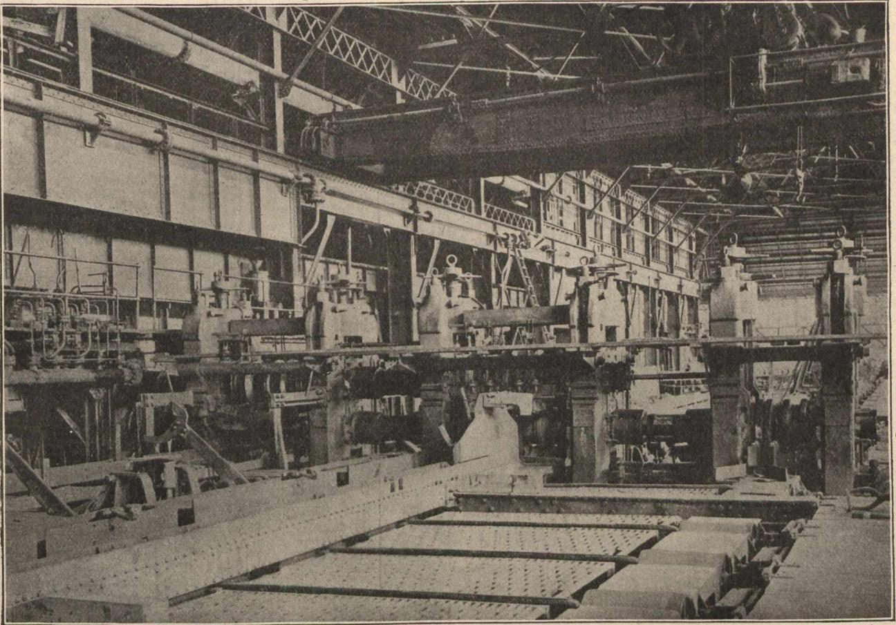
View of the Front Side of the Three Roll Trains Showing Pulpit and Transfer Arrangement.
