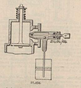
having been intimately penetrated by a current of air, this spray is volatilized by the heated surfaces and then fed to the motor.
