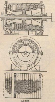
casing with V-shaped ports, which are so arranged that the ports in any three consecutive rings are never in com-munication at one time. The other end of the machine is provided with rings on the cylinder, and rings on the casing, with V-shaped ports reversely arranged to those on the forward end.
