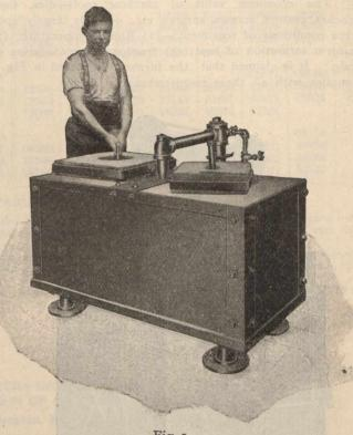
Fig. 1. Hardening High Speed Tool Steels.
