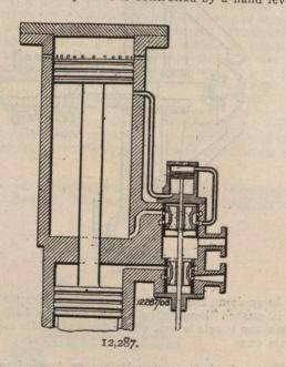
has heretofore been necessary where a number of repeated blows was desired, to move the lever at each stroke. By the present invention such lever may be switched out of action, and the hammer caused to work automatically and continuously.
