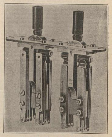
Fig 2 .- Two-way Listening and Two-way Ringing Key.
