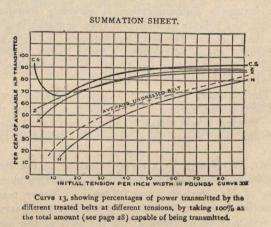
engine used had a limit of 40 R.P.M. per minute, the load being applied by means of a pony brake. As will be seen from the chart, the test proved conclusively that it is perfectly feasible to run belts loose, which means increased life for the belt, no slip, no burning of the belt, less wear in journals, less lubrication, less straining of shafting and pulleys, and more available power, few or no stoppages for repairs, and loss in time and product.
