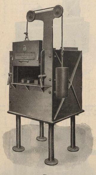
Fig. 3. Case Hardening and Annealing Furnace.
