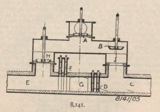
chimney, and, having passed through the dampers F F, proceed by the flue G, keeping always in the same plane or level.
