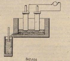
carburizing a metalliferous substance is done by fusing it as an electrode in presence of a substance having a high affinity for carbon.
