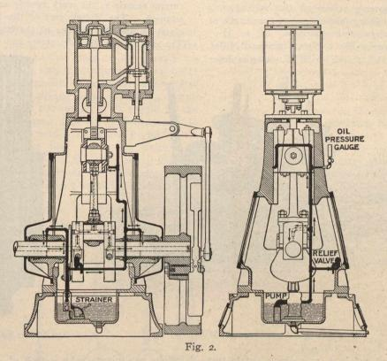
Showing System of Forced Lubrication, Watershed Partition and Enclosing Frame.
