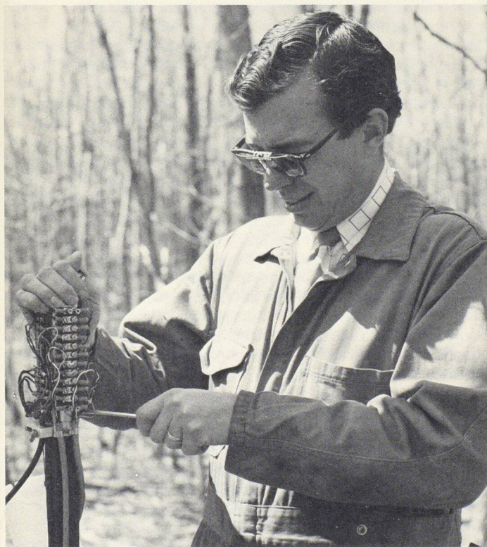
Dr. Michael Watson makes an adjustment to the main terminal box linking the four infrasonic microphones.
