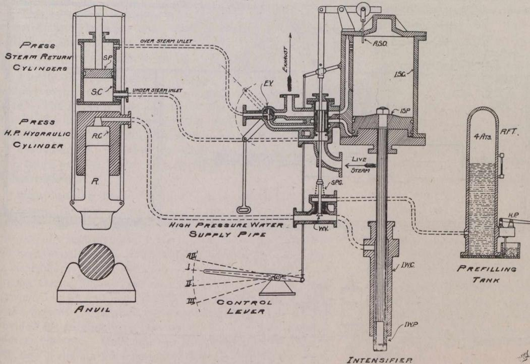
**Diagrammatic Sketch of Steam Hydraulic Press, showing the operating cylinder and valve systems with single control lever.**
