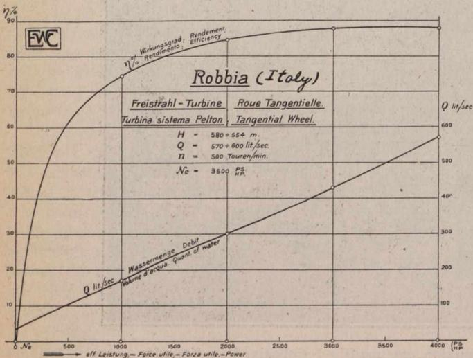
only rose to a very few per cent. above normal. The above efficiency curve which exceeds the guaranteed figures by about 8 per cent. is remarkable by the fact that it remains above 80 per cent. from over-load to one-quarter load. A general description of this plant was given in The Canadian Engineer of August 31st, 1911, where full details of the installation were given.
