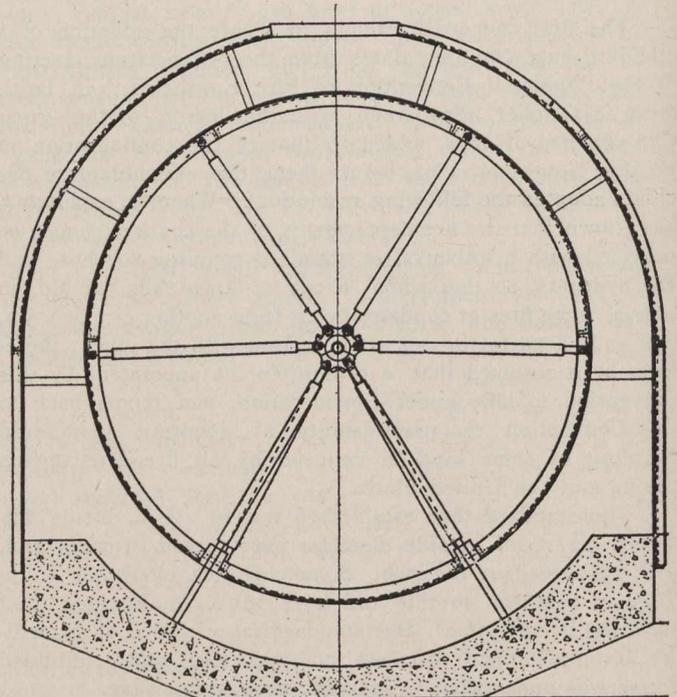
Fig. 2.—The System Used for Building Large Concrete Pipes.
