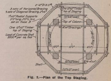
The shearing stress per square inch is  $6400 \div 12 \times 9.7$ = 55 lb. The compressive stress per square inch is 10,800  $\div 12 \times 8 = 113$  lb., showing also an unusually high factor of safety.
