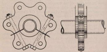
Fig. 3.-Cast Iron Collar on Central Horizontal Shaft,
