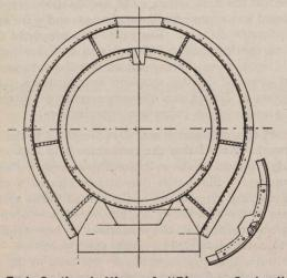
Fig. 1.—End Sectional View of "Blayney System" Collapsible, Telescoping Steel Forms and Centering.
