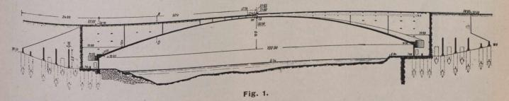
to the remarkable dimension of 8-in. (20 cm.), from this point it has been increased until it is 20-in. (50 cm.) at the springing lines. The bridge is materially strengthened by 8-in. thick stiffening ribs, which extend its whole length, and over the abutments. These consist of the above-mentioned ribs connected by cross walls and supported by concrete columns, (Fig. 2 and 3), constructed in the following manner.
