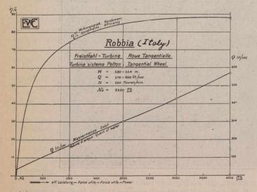
only rose to a very few per cent. above normal. The above efficiency cu.ve which exceeds the guaranteed figures by about 8 per cent. is remarkable by the fact that it remains above 80 per cent. from over-load to one-quarter load. A general description of this plant was given in The Canadian Engineer of August 31st, 1911, where full details of the installation were given.
