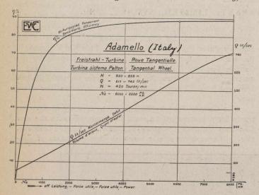
feet, each unit being designed for a maximum power of 6,600 B.H.P., when running at a speed of 420 revolutions per minute. These turbines are all of the Escher Wyss Company's special design and patent, fitted with deflecting nozzle which eliminates the employment of any relief valve, at the same time keeping the rise of pressure in the penstock remarkably low. As a matter of fact, when tests were made and the full load was thrown off, the pressure at the end of the penstock
