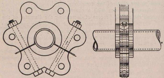
Fig. 3.—Cast Iron Collar on Central Horizontal Shaft.
