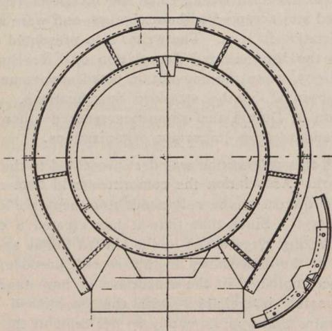
Fig. 1.—End Sectional View of "Blayney System" Collapsible, Telescoping Steel Forms and Centering.
