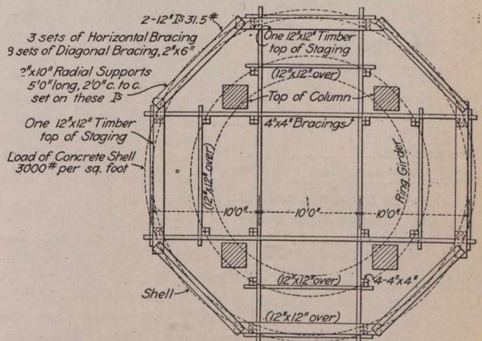
Fig. 2.—Plan of the Top Staging.
