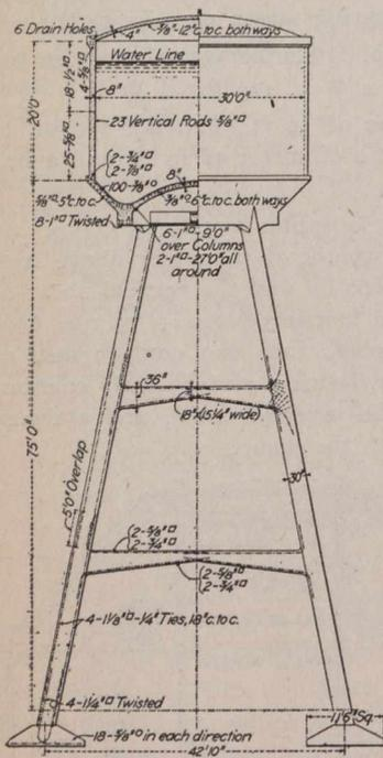
Elevation of Standards and Part Section Through Tank Showing Reinforcement.
