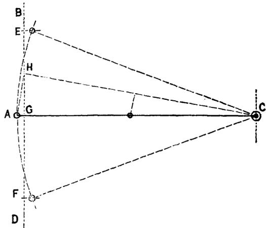
Let **C** be the centre of the walking-beam, **BD** the line of the stroke, and **EF** the length of the stroke.
