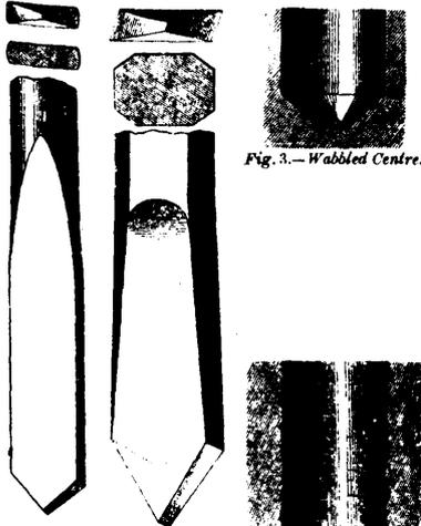
Fig. 1.—Good. Fig. 2.—Bad. Fig. 3.—Wobbled Centre. Fig. 4.—Ridged Hole.
