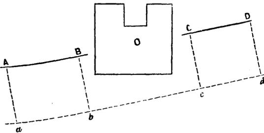
Let **AB** be the given straight line, terminated by an obstacle **O**, but required to be continued on the other side of the obstacle, as **CD**.
