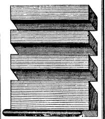
Fig. 2.—Section of Blind.
