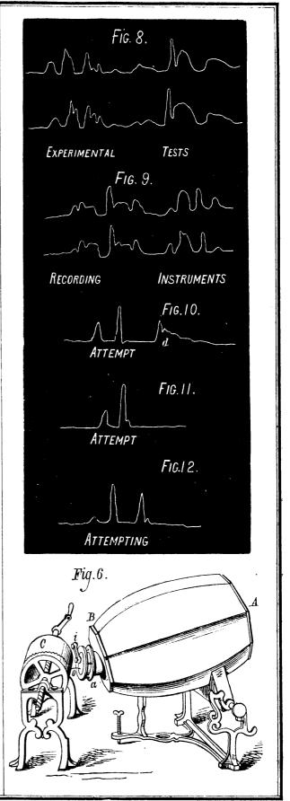
stopped by a membrane of goldbeater's skin or thin gutta percha. Against this membrane a spring presses lightly and has connected to it a light arm of aluminum, which carries a marker consisting of a very fine sable hair pencil, projecting from the lower end of a glass tube containing coloring material, the tube and pencil together forming a kind of fountain marker,
