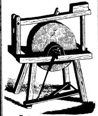
Fig. 1.—TRURING A GRINDSTONE.
