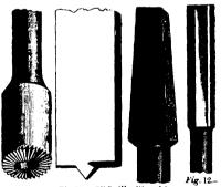
Fig. 9.—Rose Fig. 10.—Til Drill Fig. 11.— Round Cutter for Pin Square Tapereo Parallel Shank.
