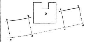
Let A B be the given straight line, terminated by an obstacle O, but required to be continued on the other side of the obstacle, as C D.
