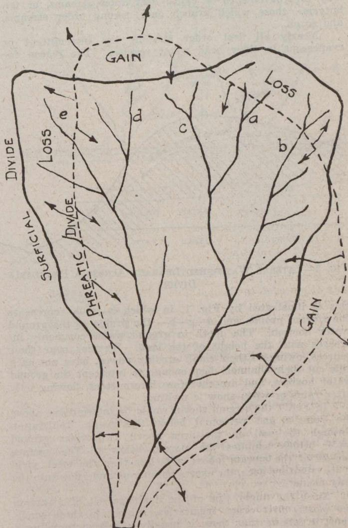
FIG. 2—CONDITIONS FAVORING WATERSHED LEAKAGE
