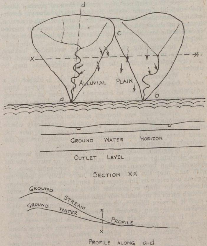
FIG. 6—CONDITIONS SUITABLE FOR WATERSHED LEAKAGE UNDER AN ALLUVIAL PLAIN
