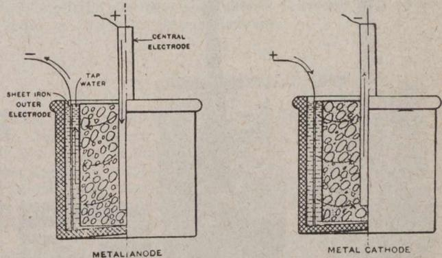
FIG. 2—METHOD OF MAKING CONNECTIONS TO SPECIMENS
