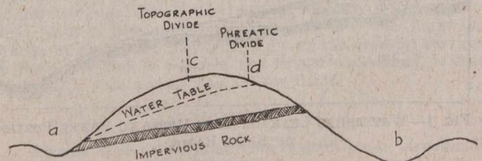
FIG. 4—LATERAL WATERSHED LEAKAGE INDUCED BY DIP OF IMPERVIOUS ROCK
