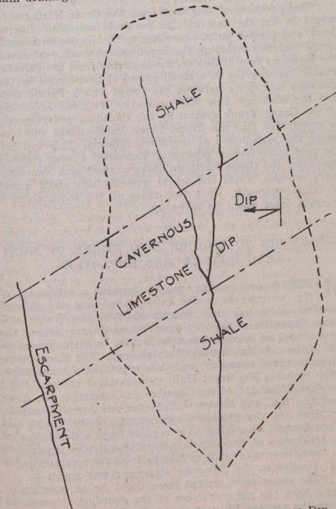
FIG. 5—WATERSHED LEAKAGE RESULTING FROM DIP, PERMEABLE STRATA
