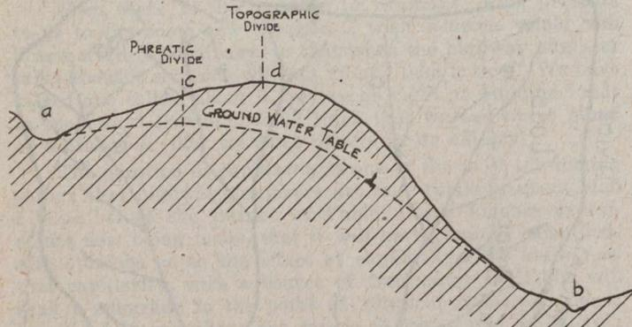
FIG. 3—LATERAL WATERSHED LEAKAGE ACROSS A PERMEABLE DIVIDE
