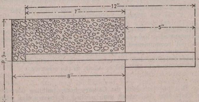
FIG. 1—GENERAL TYPE OF SPECIMENS USED
