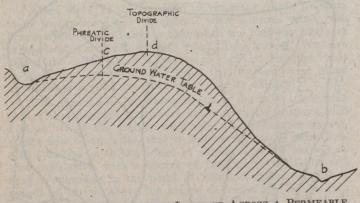
FIG. 3—LATERAL WATERSHED LEAKAGE ACROSS A PERMEABLE DIVIDE
