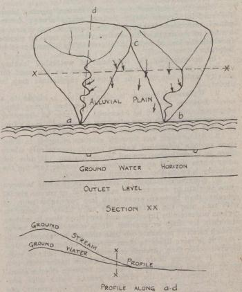
FIG. 6-CONDITIONS SUITABLE FOR WATERSHED LEAKAGE UNDER AN ALLUVIAL PLAIN
