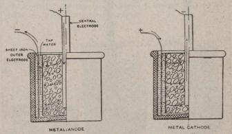
FIG. 2-METHOD OF MAKING CONNECTIONS TO SPECIMENS
