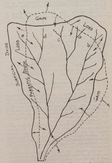
FIG. 2—CONDITIONS FAVORING WATERSHED LEAKAGE Arrows indicate direction of flow of ground water.
