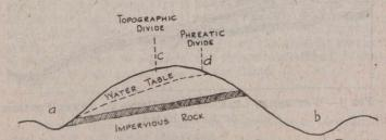
FIG. 4—LATERAL WATERSHED LEAKAGE INDUCED BY DIP OF IMPERVIOUS ROCK
