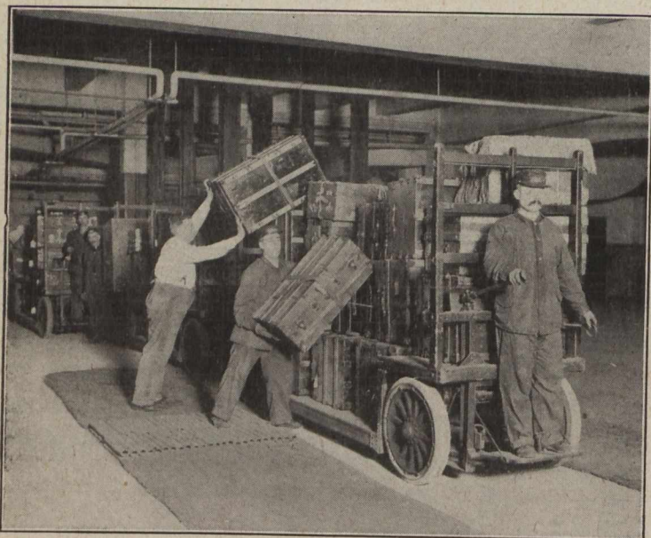
Fig. 3.—Electric Baggage Truck, for Use on High Platforms. (Note Rubber Mat of Old Hose Pipe to Protect Baggage and Flooring.)
