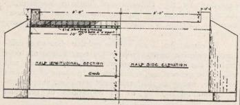
Half Longitudinal Section and Side Elevation of Concrete Culvert over Sullivan Creek, Essex County, Ont.
