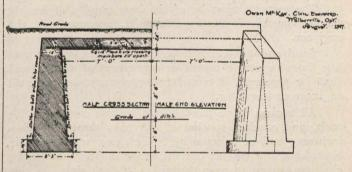
Half Section and End Elevation Concrete Culvert over Sullivan Creek, Essex County, Ont.
