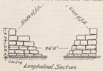
always be taken to secure good, firm bottom, and the foundation course should be placed well below the bed of the stream, and thus prevent undermining of the walls.
