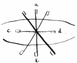
The function of our rudders ("balancing rudders"?) is to turn the machine around a longitudinal axis as desired, without turning it around a vertical axis.
