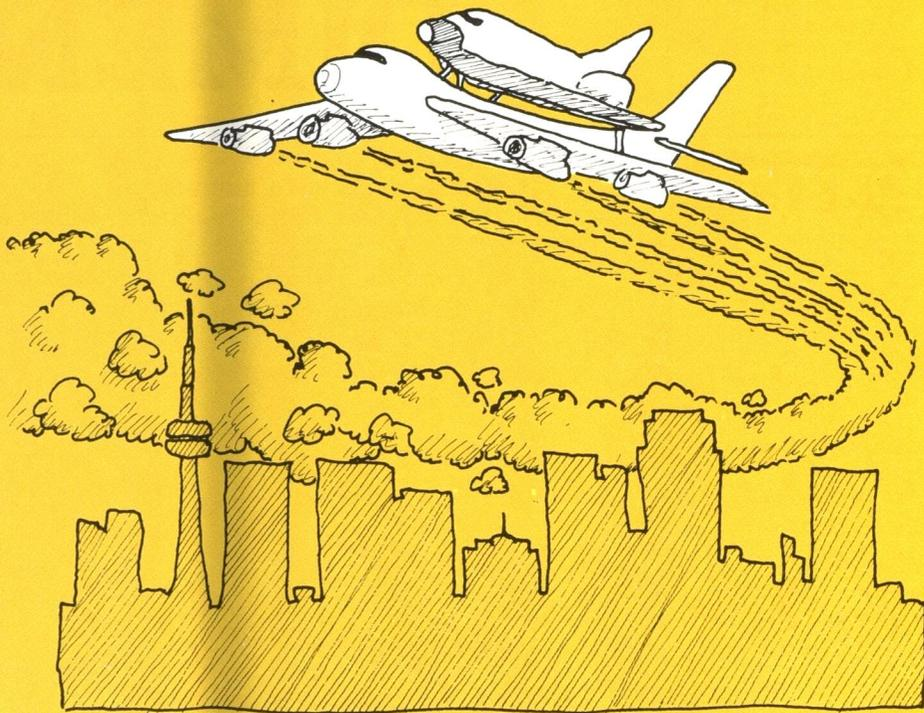
Space shuttles, verging on the size and weight of a medium commercial jetliner, do not encourage hang glider flying methods. Yet in effect, that is just what the *Enterprise* accomplished in 1977, when it detached from the 747 transporter and returned safely to the sands of Edwards Air Force Base in Southern California. In the course of the test series, the 37-m, 68 000-kg vehicle made five successful powerless flights to pave
