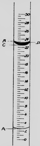
Fig. E. Measuring the fat column in the neck of a cream bottle. Reading should be made from A to C, not to B or D.
