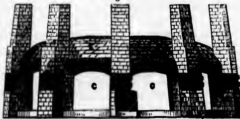
Elevation.—A, Elevation of Sieve above the Glass-house Floor. BB, Flues above the Pillars. CC, Openings for Crucibles. D, Furnace Door. E, Reverberating Dome.
