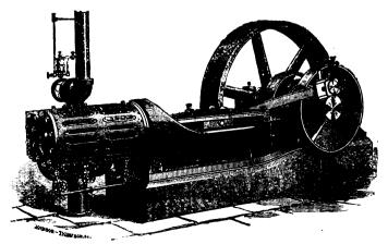
Manufacturers of the Celebrated ARMINGTON and SIMS AUTOMATIC CUT-OFF Steam Engine from 20 to 200 Horse Power, built for heavy and continuous working, and adapted to any required speed. Close regulation and best attainable economy of fuel guaranteed.
