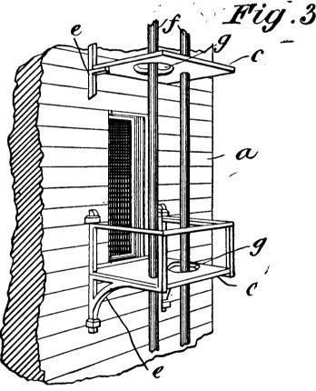
floors or staging from the roof to the ground; g g are circular openings which alternate from one side to the other at each succeeding landing. The landing to be placed before a window at every story.
