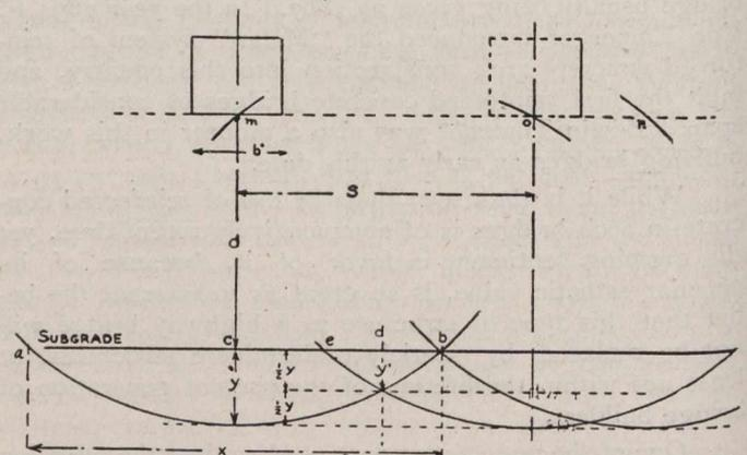
**Fig. 2.—Width of Load Distribution Graphically Expressed.**
