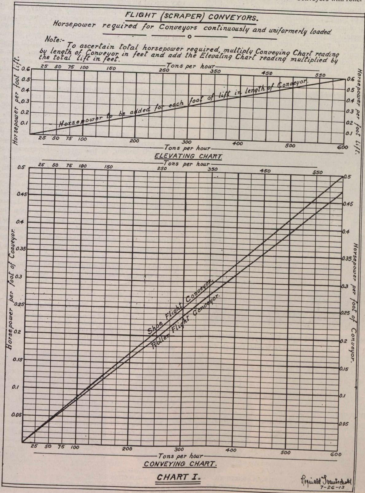
Horsepower required to convey load.
