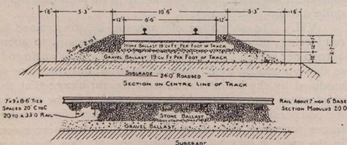
**Fig. 1.—Track Superstructure for 60,000 lb. Axle Loads.**
