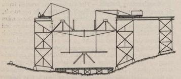
Fig. 8.—Method of Hoisting and Erecting Trusses.
