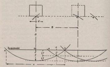
Fig. 2.—Width of Load Distribution Graphically Expressed.
