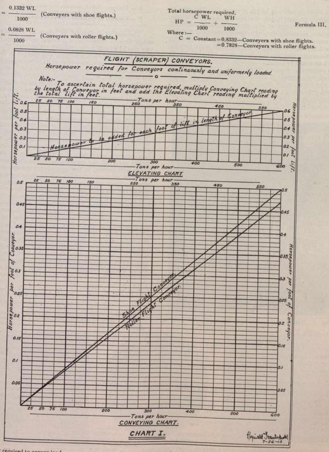
Horsepower required to convey load.  $HP = \frac{W' \ge 0.7 \ge V \ge L}{33000} = \frac{0.7 \le WL}{1000}$ Horsepower required to elevate load.  $HP = \frac{W' \ge V \ge H}{33000} = \frac{WH}{1000}$
