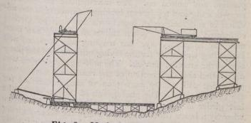
Fig. 6.-Method of Moving Tower.
