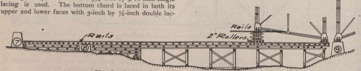
Fig. 5.-Staging Track for Moving Towers Into Place.
