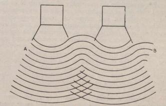
Fig. 4.-Lines of Distortion of Ballast Under Loaded Ties
