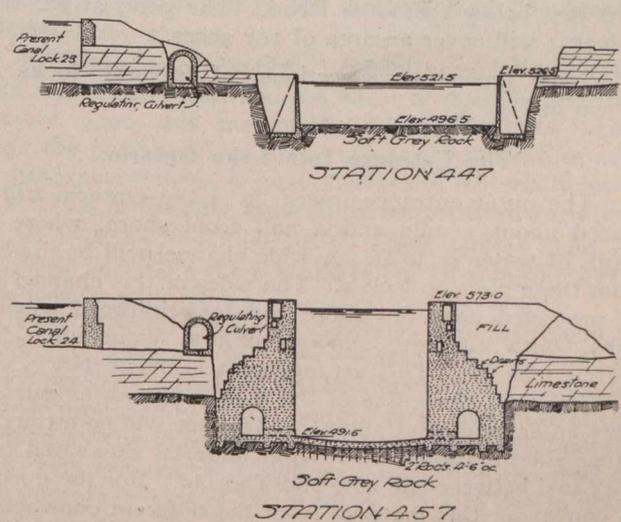
Fig. 3.—Typical Cross-Section of Earth-Works at Various Points.
