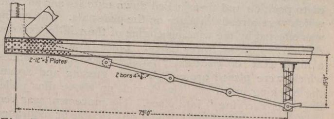
Fig. 7.—Method of Bolting and Trussing Bottom Chord for a One-Piece Erection.
