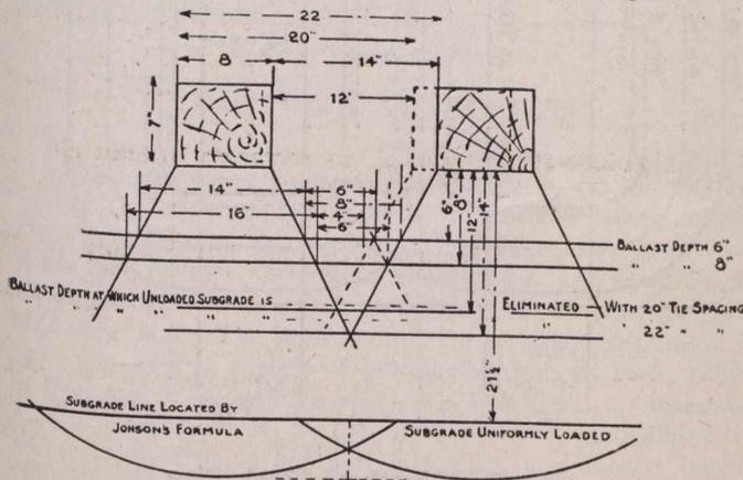
Fig. 3.—Section of Standard Main Line Track.
