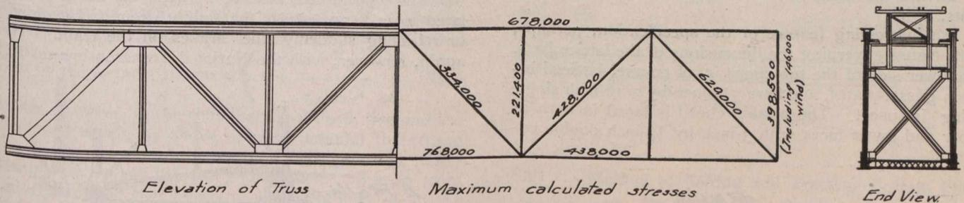
Fig. 3.—The 150-Foot Span Truss and Maximum Stresses.
