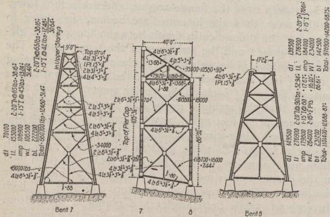
Fig. 4.—Typical Compression Stresses.
