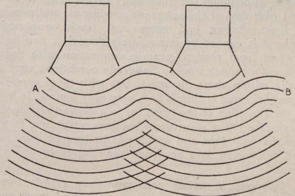
Fig. 4.—Lines of Distortion of Ballast Under Loaded Ties
