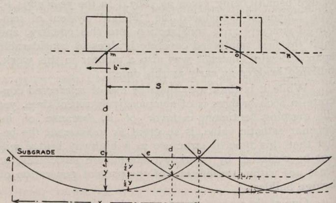
Fig. 2.—Width of Load Distribution Graphically Expressed.
