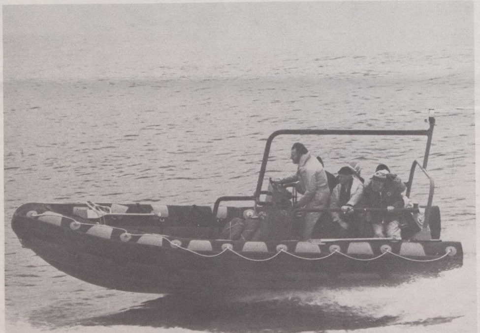
A semi-inflatable rescue boat suitable for Arctic and offshore oil exploration. The craft can endure temperatures as low as -55 degrees Celsius.
