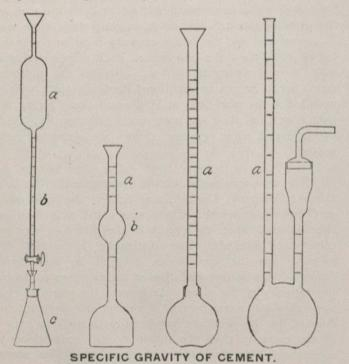
These are the various forms of apparatus now in common use for taking the specific gravity of cement. Fig. 1 is the Jackson Apparatus; Fig. 2 is the Le Chatelier; Fig. 3, the Schumann; and Fig. 4, the McKenna.
