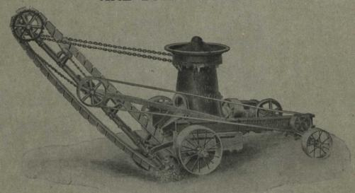
AUSTIN GYRATORY CRUSHER ON TRUCK WITH ELEVATOR.
