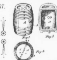
FIG. 1 is an exterior view of Cask. FIG. 2 is an interior perspective view of one section of the Cask. FIG. 3 is a transverse sectional section through middle of Cask.
