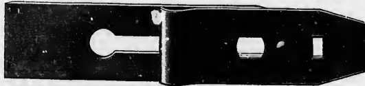
Illustration of plane iron, with cap screw moved to back end of the slot, and in position for sharpening the iron, without removing the cap.
