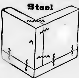
Fig. 10 shows its use in making boxes. Its application makes a much finer, stronger box and at much less expense than by the use of nails or screws.
