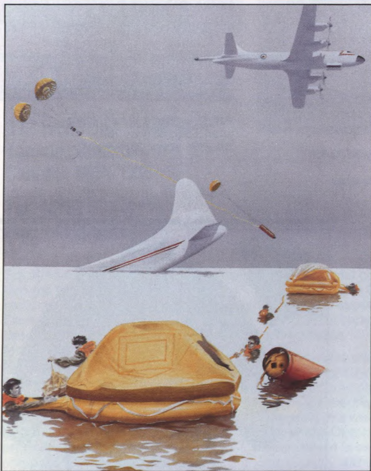
The sea SKAD survival kit being air delivered to survivors from a CP-140 Aurora (P-3 Orion) aircraft.
