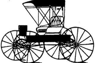
Sidespring Road Wagon—Wheels, Sarven pattern, 3/4 in. tire; Axle 15-16 in.; Painting, body black, gear, green; Seat roomy with solid back and spring cushion. Trimmings, imitation leather, with carpet in bottom of box. With shafts only..... 55.00
