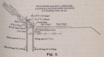
Slips.—The term, "slips," as the conventional name indicates, is applied to places where the soil slides into the river. These slips occur when the roadbed is constructed on a fill, ranging in depth from 5 to 10 feet, across narrow flats, between the hill and the river. Due to the constant movement of the earth, no trees grow on the land between the river and the railroad. The ground slips gradually into the river where, from time to time, its toe is cut away by the current.
