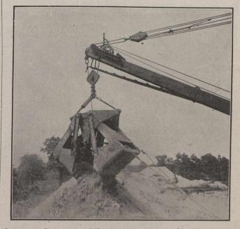
the scoops by means of the four two-part closing chains seen in the illustrations.
