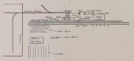
engine supplied power for the mixer and for a hoist to operate the elevator. The large panorama photograph shows very distinctly the arrangement of the industrial track for delivering concrete to the work.
