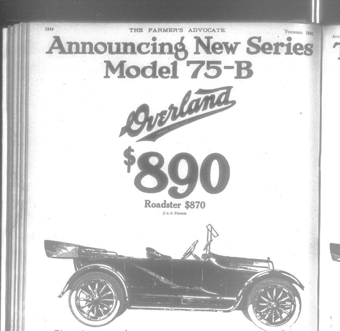
This newest Overland is the world's most powerful low-priced car. It has a 31½ horsepower en bloc motor that is a perfect marvel for speed, power and endurance. By increasing the bore of the motor from 3<sup>''</sup> to 3<sup>3''</sup> we are able to offer a power plant which at 1950 R.P.M. develops full 31<sup>1</sup>/<sub>2</sub> horsepower.
