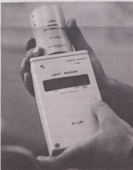
The meter designed and developed by the laboratory to record the number of hours lights are on in a room.
