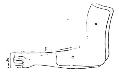
Figure 2.—Shows the hand midway between pronation and supination, the leather cap laced round the carpus and metacarpus, the cords attached to the cap and passing towards the axles to which they are also attached. The axles are hidden, but their axes correspond with the centre of the ratchet wheels. The catch and spring which prevent the ratchet wheel and axle from turning backward, are also seen, and the levers or cross handles attached to the axles.
