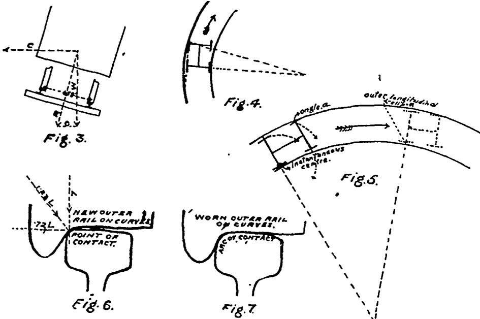
It will be seen by Fig. 5 that the truck is turning continually around the inner rear wheel as a centre, and the aggregate slippages are as follows:
