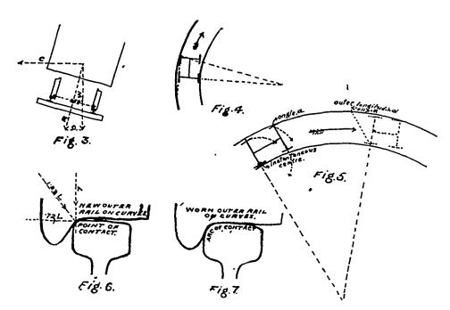
It will be seen by Fig. 5 that the truck is turning continually around the inner rear wheel as a centre, and the aggregate slippages are as follows:
