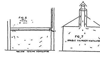
the warm room would increase in temperature so much that very little heat would be lost by changing the atmosphere of the room twice an hour (see fig. 6). By this method the extractor would have to be so arranged that it would have a keen draught.
