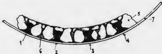
Fig. 21. 1, 2, 3, 4. Rails. 5 Quartz. 6 Mortar. 7. Shell
