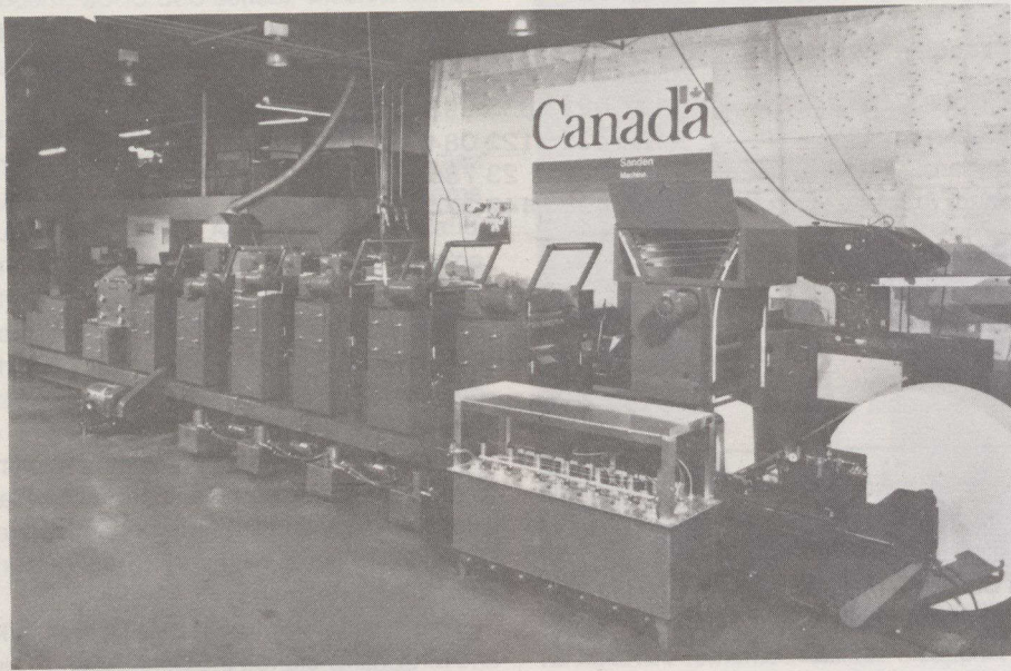
This variable size press from Sanden Machine Limited of Cambridge, Ontario requires only a pull on a lever to make it the fastest available today for size changeover.
