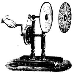
Fig. 4.—Recomposition of white light by means of a rapidly revolving disc, colored in sectors.
