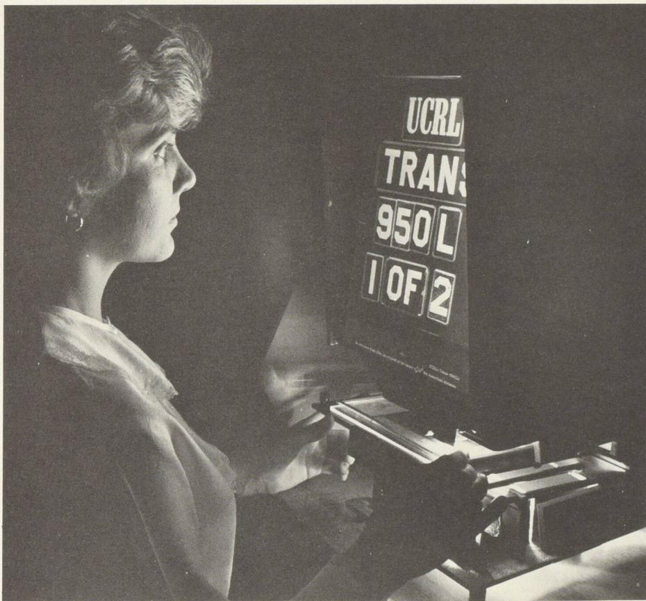
*Many research reports are filed at the NSL on film cards known as microfiches. Each card contains up to 60 pages of printed material. Operator uses a microfiche reader to enlarge printed material and project it on illuminated screen.*
