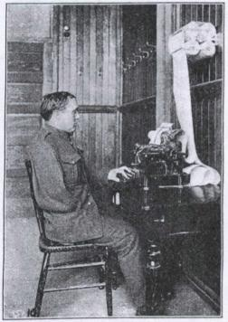
Feeding device for typewriter operated by man with one arm.
