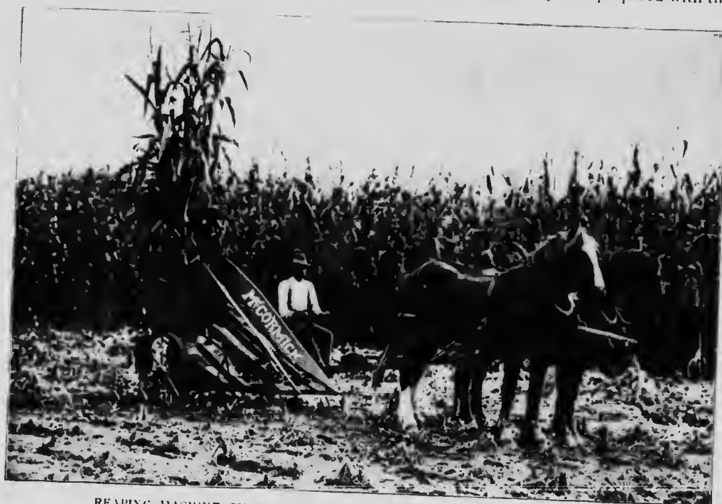
REAPING MACHINE CUTTING OFF STEMS AND BINDING THEM INTO SHEAVES
