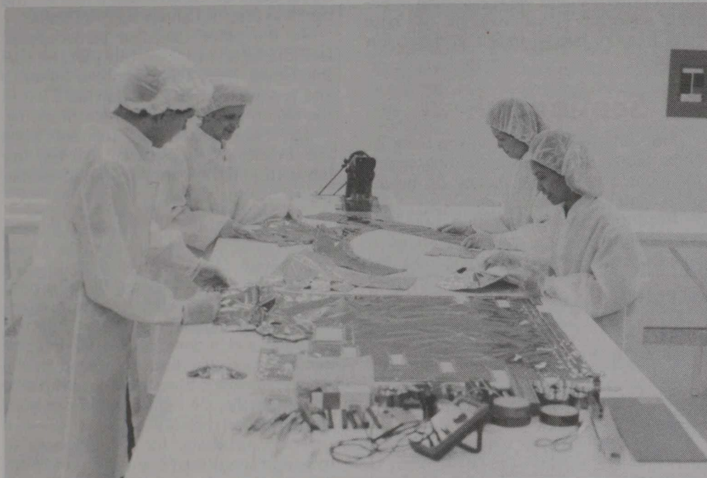
Fell-Fab clean-room solar blanket production for the European satellite program.
