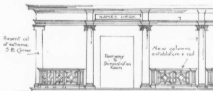
This illustration shows the front elevation of the colonnade that is to be built out to the front of the stands. The opening is directly in front of the entrance to the sound proof room at the rear.
