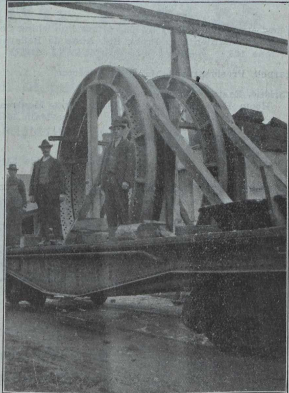
Four giant tread rings 14 feet in diameter moulded in on piece with gear moulding machine, combined weight 30 tons.
